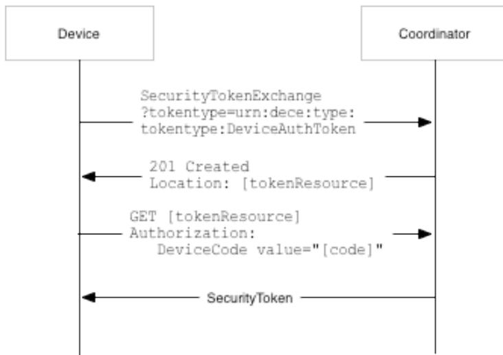
Figure 4: Device Authentication Token Exchange
