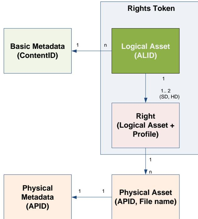
A Logical Asset is identified by an ALID. There are up to two profiles (SD and HD) that may be associated with that ALID. Technically, the Discrete Media image is not a profile, but in terms of information management it is treated as such. The combination of Logical Asset and Profile are referred to as a Right. Rights are maintained in the Rights Token.
