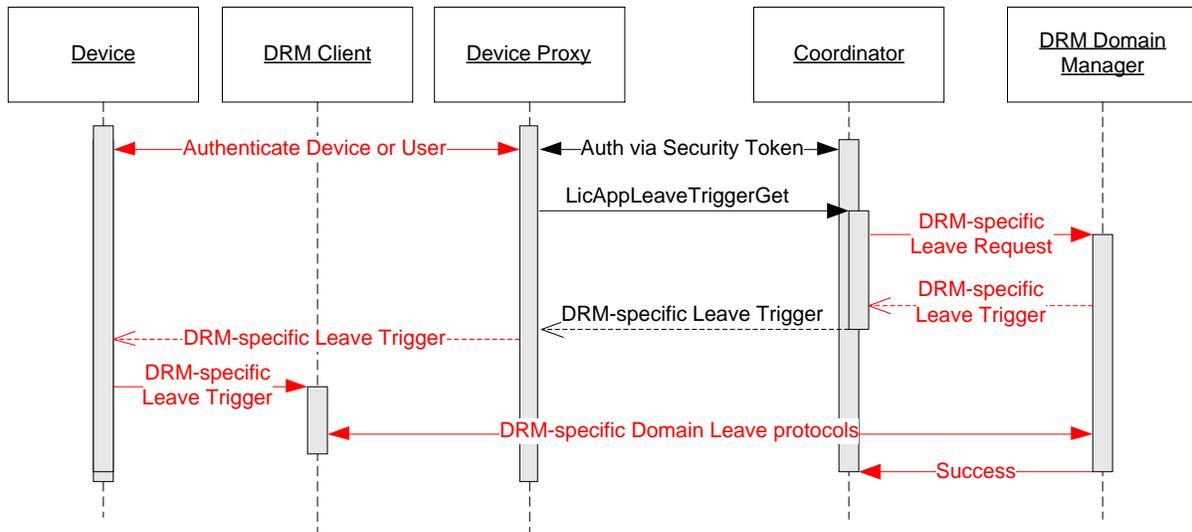
**Figure 20 – Device Proxy Initiated Device Leave (illustrative)**
