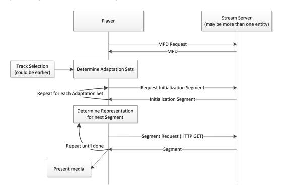
Content protection processes such as obtaining a license is required for some content. When Common Encryption is used, a license is generally obtained following Track Selection and prior to presenting media.
